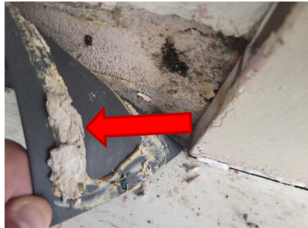
Brown mastic on black vinyl baseboards does not contain asbestos (S-004A-C).
