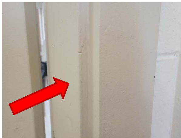
Brown paint on wood door frame contains <0.0005% lead (LP02).
